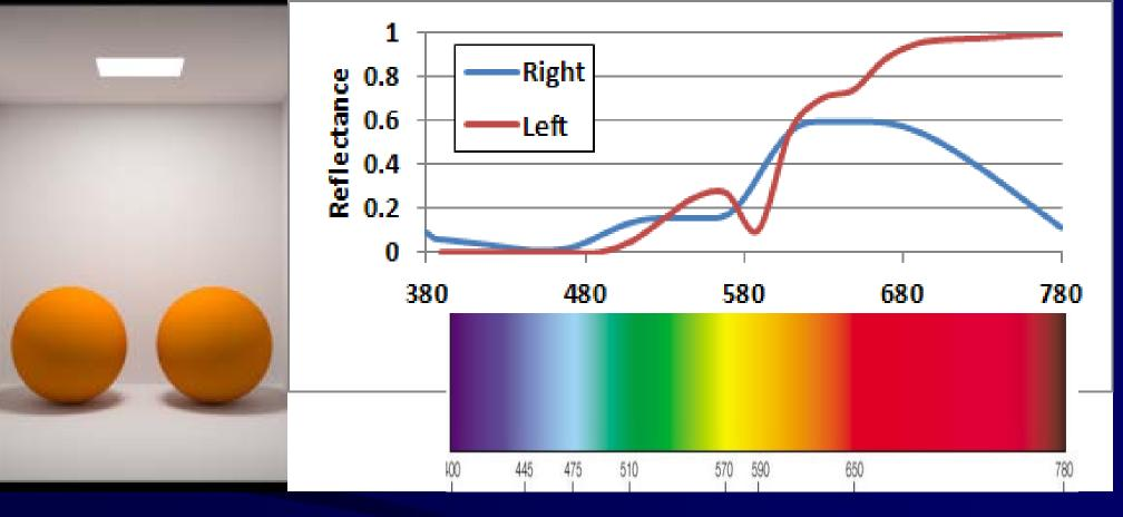
The two YO surfaces look identical under daylight, but each surface is actually reflecting a different spectrum of colors. The left sphere has stronger red reflectance and no blue. The right sphere has modest red, strong orange and a bit of blue and green. To our tri-stimulus eyes, these traits "average" to the same color – the spheres look virtually identical. Tuorescent
