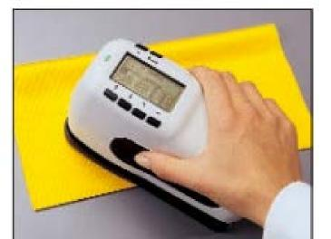
A portable sphere spectrophotometer measures the color of textile samples and other materials where the product's appearance is critical for buyer acceptability.
